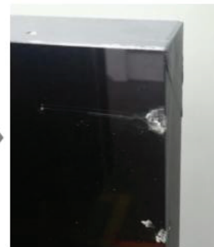
Bezel & Panel Damage
