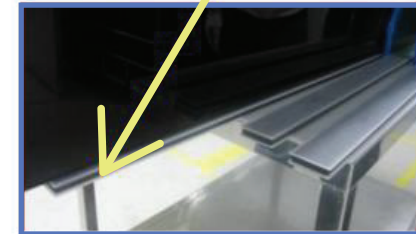
Form Pad is required to lessen shock to LCM
