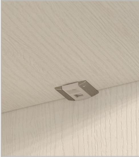
UNICO is a wood shelf support to be slotted into the panel by making face borings. It is conceived also for transportation, as the shelf is secured in position, thus it is a useful solution for both flat pack and rigid furniture. It consists of a zinc alloy shelf support with a ridged wing on both sides combined with a sliding engineering plastic clip.
