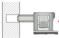
Assembling with threaded pin to achieve horizontal connection
